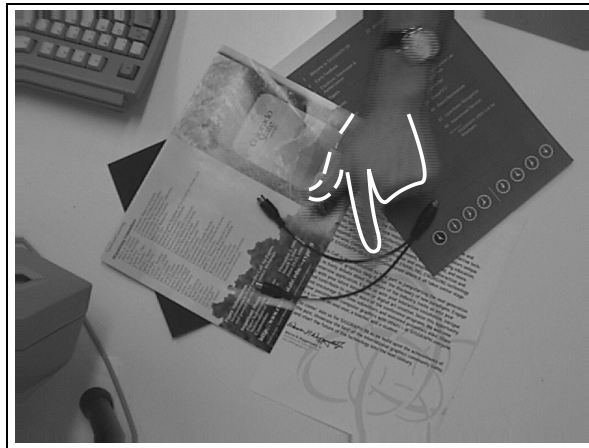
Fig. 4. Heavy clutter does not hinder the hand tracker. Even moving the papers on the desk to invalidate the background subtraction does not prevent the Condensation tracker functioning. The fingertip localisation is less robust, however, and jitter increases in heavily cluttered areas.
