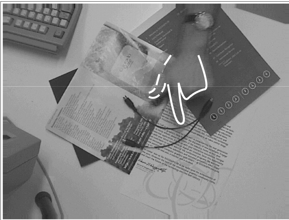
Figure 5: Heavy clutter does not hinder the Condensation tracker. Even moving the papers on the desk to invalidate the background subtraction does not prevent the Condensation tracker functioning. The fingertip localisation is less robust, however, and jitter increases in heavily cluttered areas.
