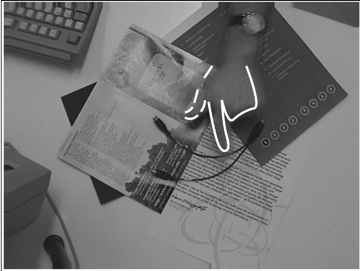
Figure 7.9: Heavy clutter does not hinder the Condensation tracker. Even moving the papers on the desk to invalidate the background subtraction does not prevent the Condensation tracker functioning. The fingertip localisation is less robust, however, and jitter increases in heavily cluttered areas.
