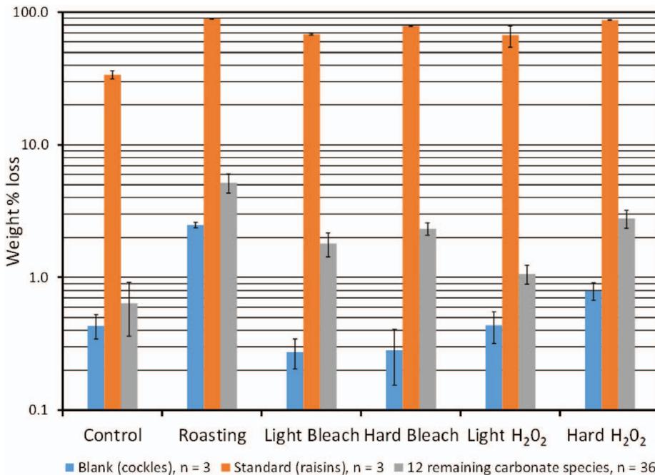
FIG. 2.—Percent weight loss by three different materials in six different treatments. Error bars are ± 1 st dev.
