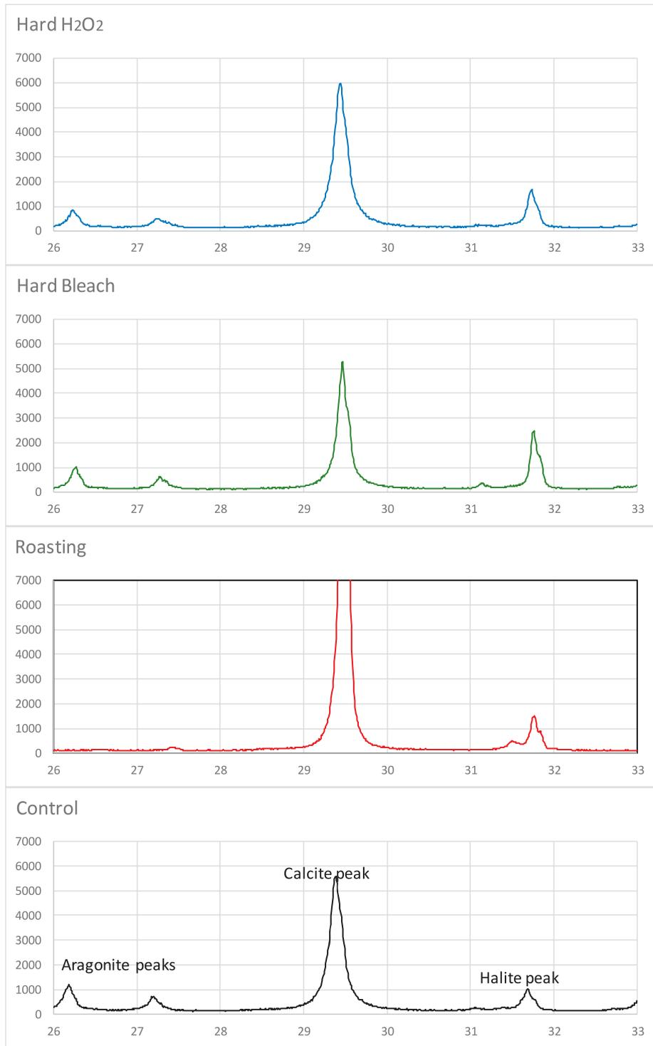
FIG. 4.—X-ray diffractograms showing carbonate mineralogy of bimineralic *Mytilus galloprovincialis* specimens exposed to various pretreatments to remove organic material. Major aragonite peaks occur at peak positions 26.2 and 27.2 °2θ (sometimes a minor peak appears at 31.1 °2θ); calcite is at 29.4 °2θ; halite internal standard is at 31.7 °2θ. Y axis is “counts.”
