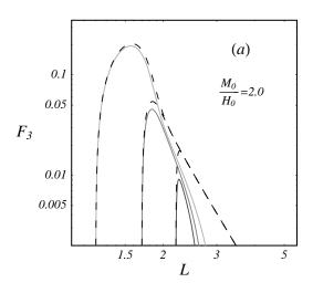
Figure 2: Force as a function of length for a particular experiment. The dashed curves represent the nonmagnetic case while the solid curves show the magnetic effects.
