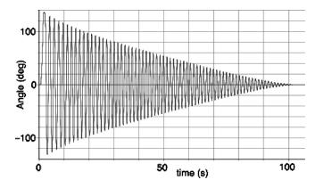
Fig. 4. The physical pendulum is displaced by an angle of  $135^{\circ}$  and released. The oscillations take just under 2 minutes to die out.
