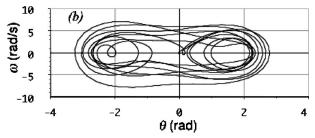
Fig. 9. (a) Rotary motion sensor data for the angular displacement of a chaotic physical pendulum vs time is shown in the top graph; (b) phase plot depicting rotational velocity vs angular position for the first 30 s of motion of the same pendulum.
