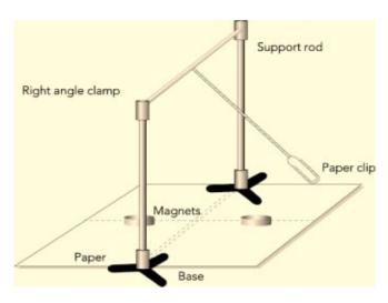
Fig. 3. This paper clip pendulum bob is reasonably insensitive to initial conditions if no magnets are present.
