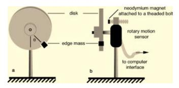
Fig. 1. The basic physical pendulum with adjustable eddy damping.
