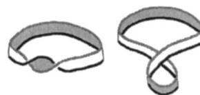
Fig. 4. A ribbon with a 360^\circ twist is equivalent to an untwisted ribbon with one crossing. Shown here is a counterclockwise twist containing helicity -\Phi^2 when measured with the helicity meter of Fig. 1. A clockwise twist contains helicity +\Phi^2 .
