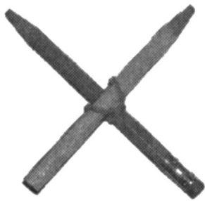
Fig. 1. A helicity meter consisting of two pencils.
