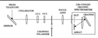
**Figure 1** Schematic diagram of the optical path through the 12-µm vector polarimeter. The beam from the telescope formed an image, was collimated, and passed through 1/2- and 1/4-wave plates and a polarization chopper. An image is then formed at the spectrograph entrance slit and the spectrum is dispersed by a grating onto the detector array.
