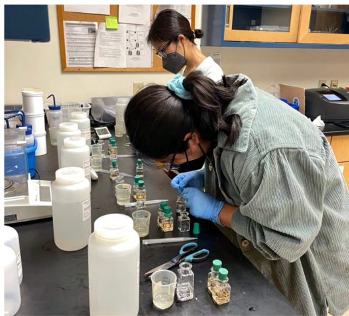
Michelle Hom (back) and Michelle Cao (front) prepare samples using the cadmium reduction method.
