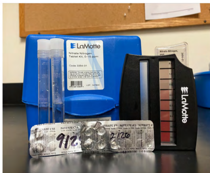
This Nitrate kit utilizes the aforementioned Nitrate #1 and Nitrate #2/CTA tablets to create a chemical reaction
