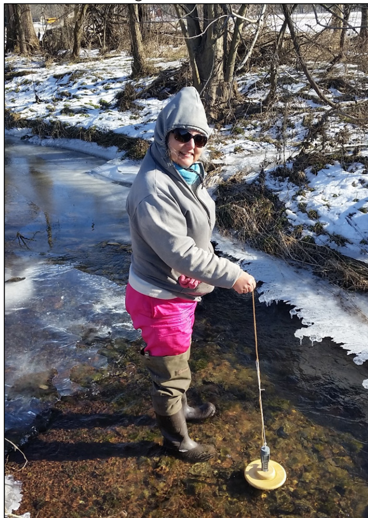
Tina Gleim (volunteer) shows off the DIY probe float which allows for monitoring without having to bend down or put hands into cold, winter waters. Photo credit to Jeff Gleim
