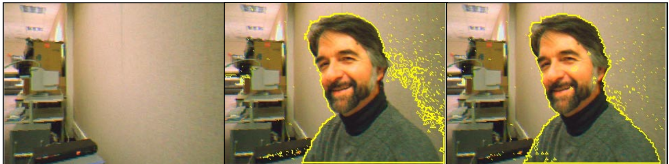
Figure 4. Left: background model image; Center foreground contours; Right: foreground after shadow suppression.
