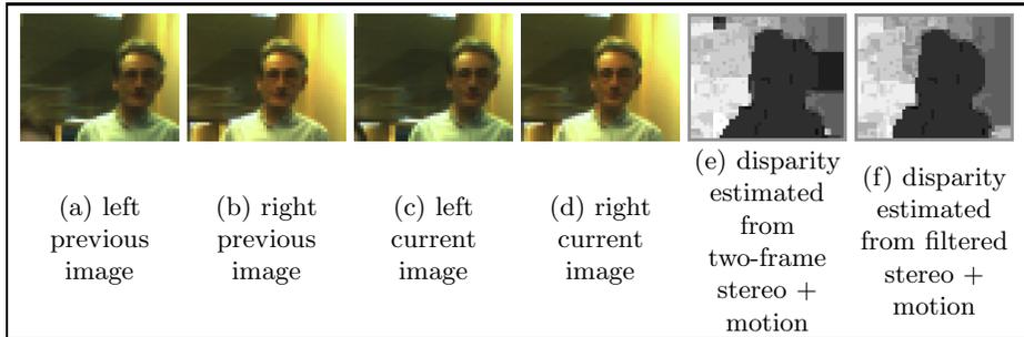
**Fig. 3. stereo+motion propagates disparity estimates through multiple frames.** The foreground person has stopped moving, and there is a large left occlusion in the textureless area on the right hand side of the image. The two-frame stereo computation (e) has no information about the disparities in this occluded region and the lack of texture causes a large artifact. The filtered stereo+motion estimate (f) propagates disparity estimates from previous frames to stabilise the difficult region.
