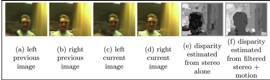
**Fig. 2. stereo+motion estimates disparity through transient occlusions.** An occluder has appeared in the bottom corner of the left current image (c) but not yet in the right (d). The stereo computation alone (e) does not have enough information to estimate the disparity in this region, but the filtered stereo+motion algorithm (f) uses information from previous timesteps to improve the result.
