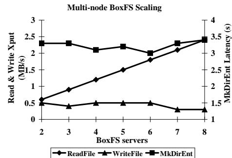
Figure 8: **Performance of BoxFS sharing experiments.** MKDirEnt Latency is the elapsed time to insert all 100 files.
