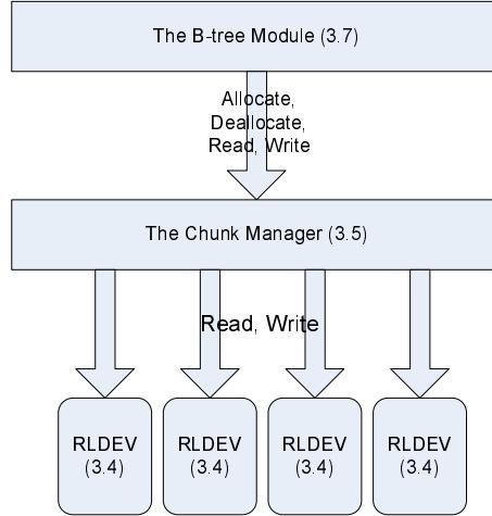
Figure 1: **Design of the Boxwood abstractions.** The B-tree is layered atop the chunk manager, which is layered on top of the replicated logical device. The numbers in parentheses refer to the section describing the design of the module.
