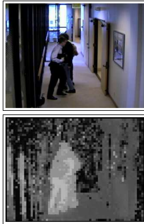
Figure 8: The foreground model cannot distinguish between three people. Two people cross in front of a third who is almost entirely obscured. A single pooled model is used for all foreground objects, so it is impossible to distinguish between different people purely on the basis of the log-likelihood ratios y_g^l shown here. Separate object models learned online might help to disambiguate between people.
