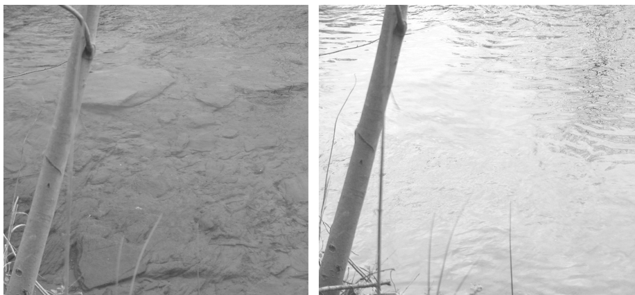
Figure B-12: The two pictures above were taken of the same scene. The picture on the left was taken with a polarizing filter, while the picture on the right was taken without a filter. What does a polarizing filter do and why does it reduce the glare from water? Why do you think fishermen often wear polarizing sunglasses?
