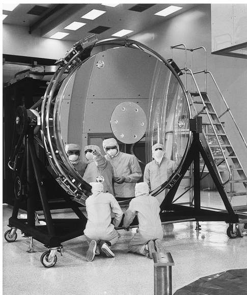
Figure B-13: The mirror inside the Hubble Space Telescope is shaped so that light entering along the axis of the telescope will be reflected to a focus at a single point. Because the mirror on Hubble is so large, it is possible to see very dim objects. (Courtesy NASA)
