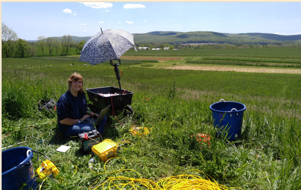
Rising Junior Ivy Gilbert is learning to collect seismic refraction data at the Dickinson College Farm. Ivy
