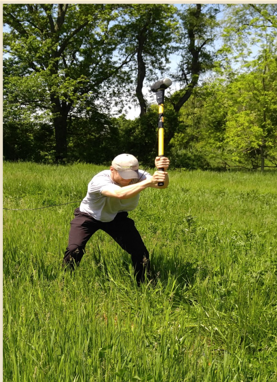
Rising senior Rob Page swinging a sledge hammer to create a seismic source at the Dickinson College Farm.
