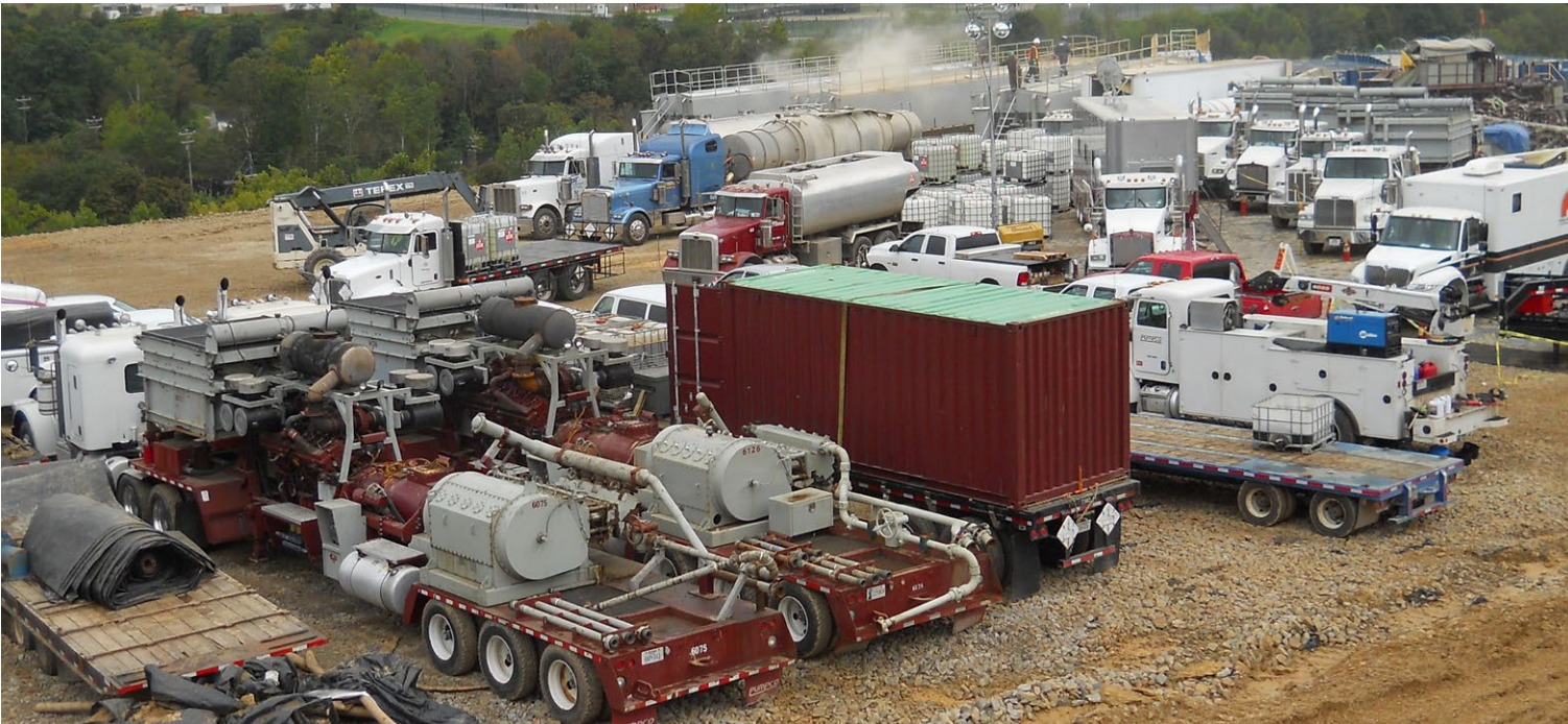
Fracking brings with it a dramatic increase in truck traffic to an area from construction to operation to water transportation. Pictured here are pumps, generators, fuel, chemicals, sand, pipes, service trucks, and other infrastructure required for the involved process of hydraulic fracturing. (Photo courtesy Doug Duncan, USGS).
