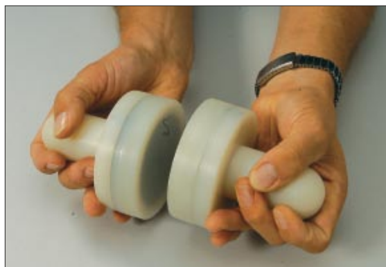
Fig. 1. An Alnico magnet and a piece of iron of the same mass are each indistinguishably encapsulated in nylon cylinders. Students can now simultaneously feel the force that the magnet exerts on the piece of iron and the force that the piece of iron exerts on the magnet.
