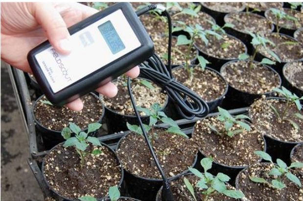
WaterScout SM 100 sensor shown with the FieldScout Soil Sensor Reader (Item 6465)
