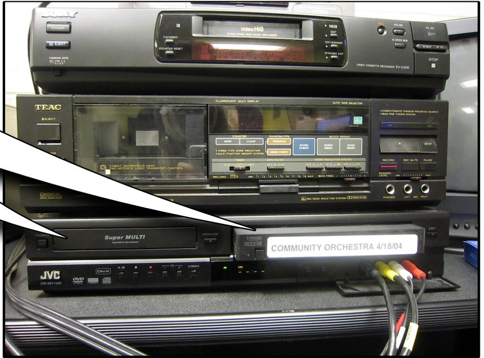
Use the AUX button on the remote until you see the tape show on the TV. The TV needs to be on AV1 Mode.
