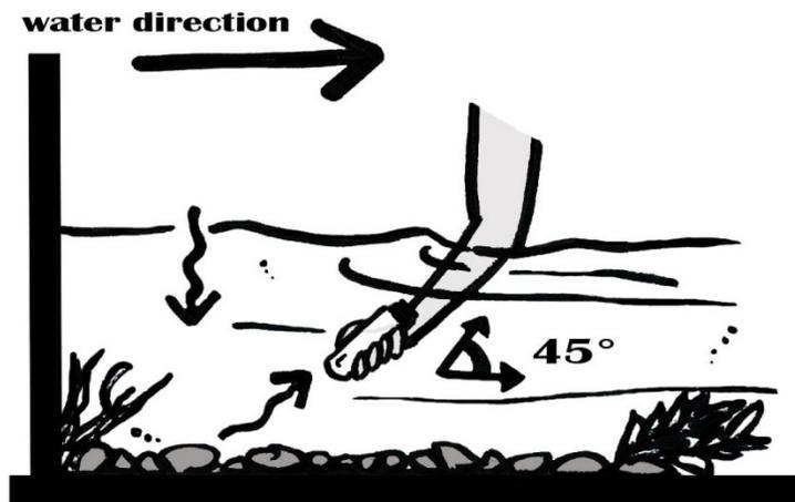
4. Lower the bottle into the stream current at an angle, attempting to smoothly and evenly sample the entire depth of the stream. Keep the same tilt to the axis of the bottle throughout the fill cycle. Keeping the sample bottle slightly tilted in this manner will prevent total filling. This empty space will allow for thermal expansion during shipping. Try to get the same volume of sample at each depth.
