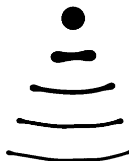
FIG. 8. Experimental results of a ferrofluid in a Hele-Shaw cell. As the magnetic field strength is increased, the finger becomes longer and thinner. The top image has no applied field and the second image from the top represents the first stable finger we found. This rather dramatic change is consistent with the first-order transition predicted in Fig. 6.
