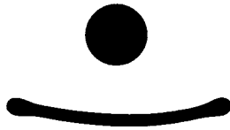
FIG. 2. Photographs of a ferrofluid droplet in a Hele-Shaw cell with no magnetic field (top) and with a perpendicular external magnetic field (bottom).
