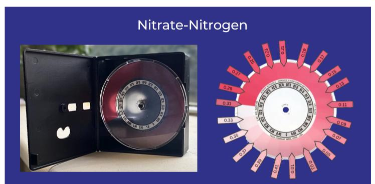
When recording values for nitrate-nitrogen, you can select the numbers shown on the HACH wheel or the values directly in between.
