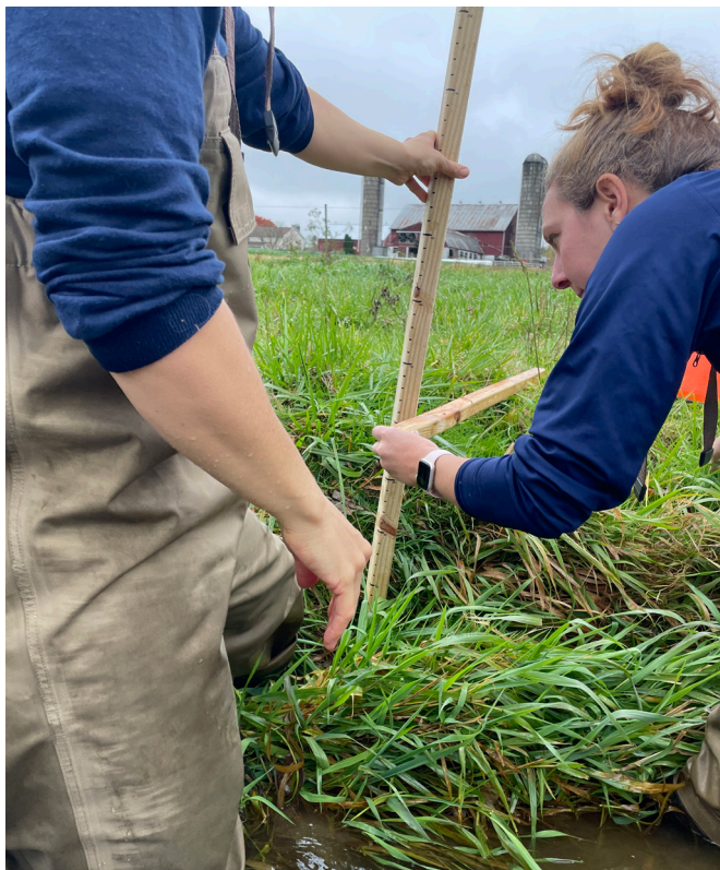
Left: Liz Chudoba (Alliance for the Chesapeake Bay) and Jules Vastine (ALLARM) troubleshoot measuring bank angle in the presence of emergent grasses. Right: Illustration created by ALLARM Outreach Manager, Phoebe Galione, to reflect this in-field troubleshooting.
